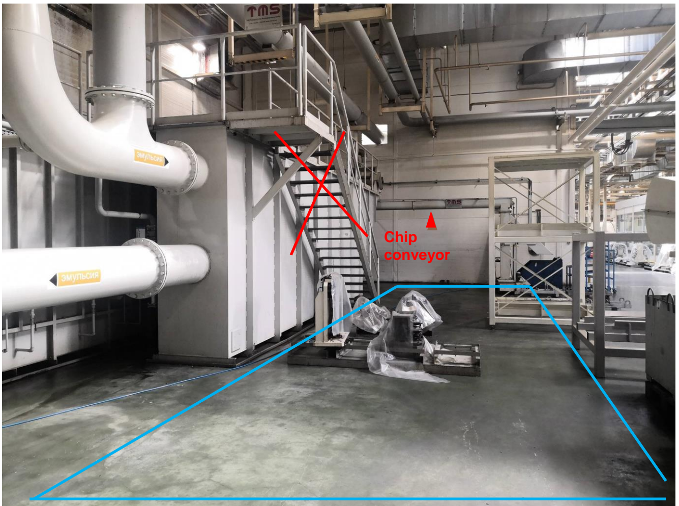
Pic.2 - possible location of the additional vacuum filter (blue color on the picture).
