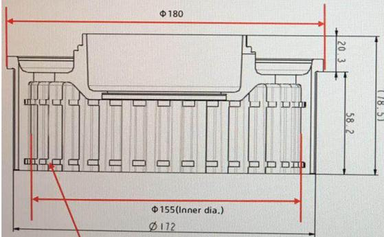
Groove and spline teeth are needed to be machined after assembling with Shaft
